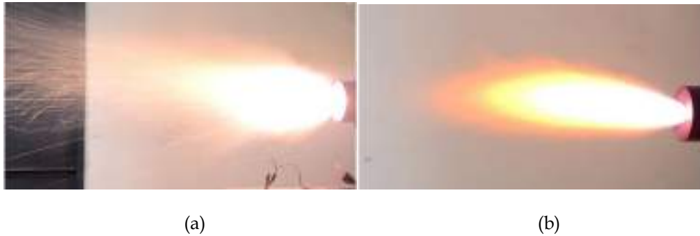
FIGURE 10. (a) Combustion test of pure paraffin and (b) combustion test of P-CB- MgB_2 [39].
